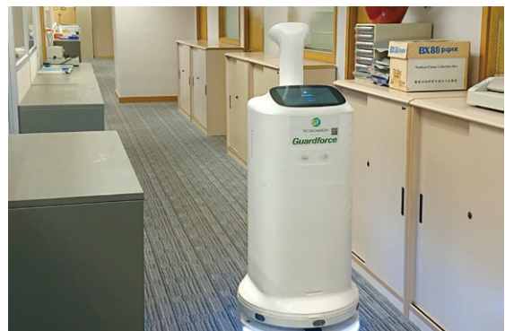
A smart robot powered by a disinfection system is stationed in the head office, which operates on auto-pilot along preset routes to spray and disinfect the premises.
